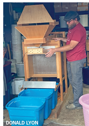
Andrew Still demonstrates the Winnow Wizard seed cleaning machine, invented locally by Mark Luterra, which is used to clean all of Adaptive Seeds' seed crops.
