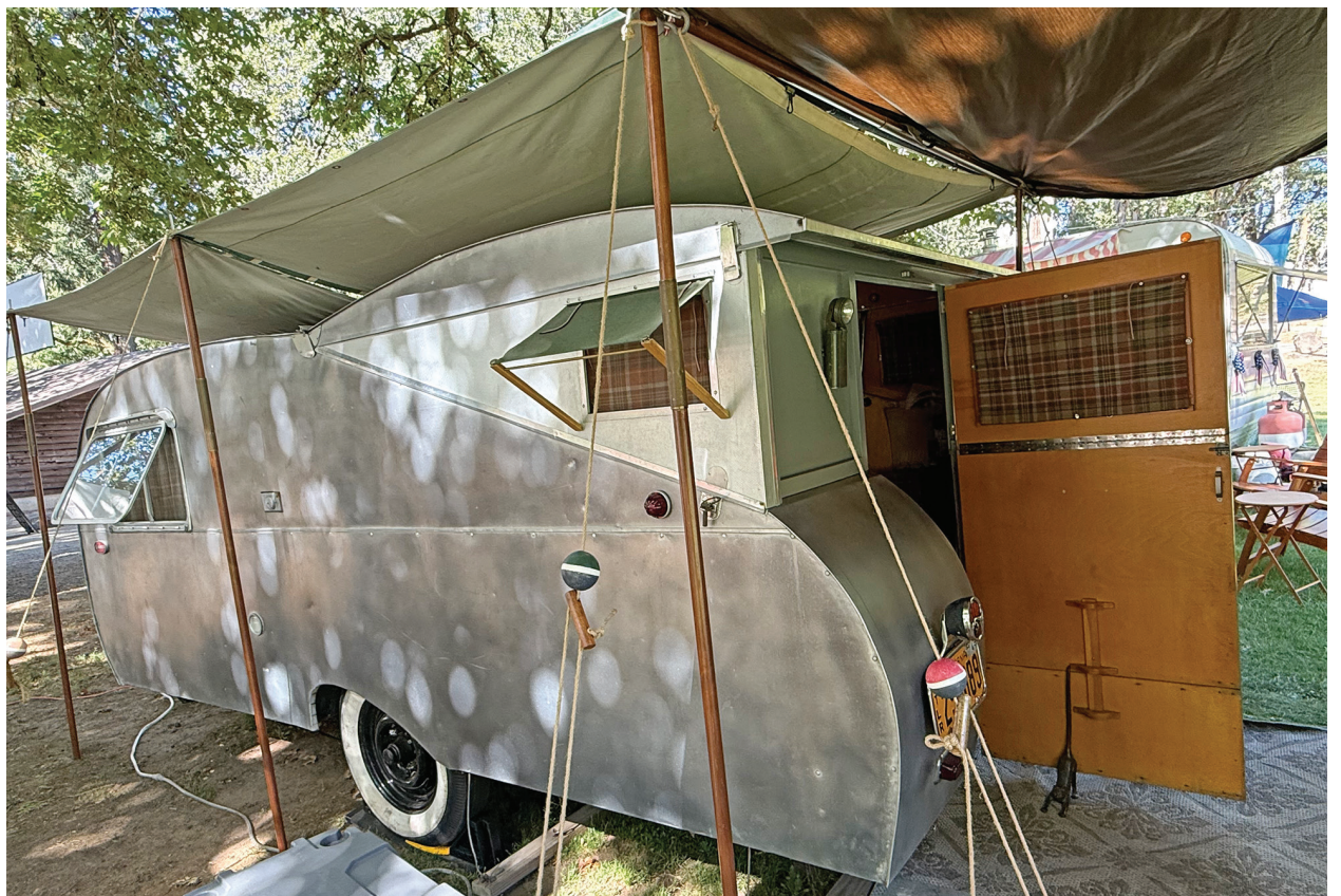
The enlarged teardrop style 1949 Zimmer "Wee Zim." is unique — when you lift the roof, the bottom center floor drops down automatically, and vice versa when lowering the roof.
